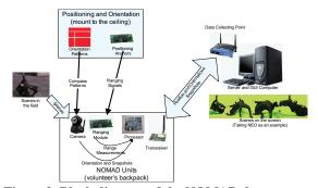
Figure 2. Block diagram of the NOMAD demo system
